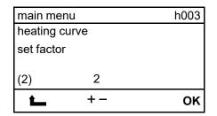
Setting range of the heating curve from **1** to **4**. Factory setting: **2** The value to be set is based on the size of the room being heated. Guide values:
