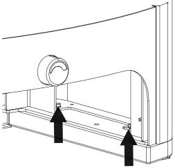
Fig. 56: Undoing the screws on the inside
