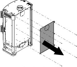
6) Remove cover with seal (1) on the back.
