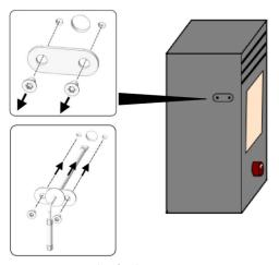
Fig. 35: Fixing the firebox temperature sensor
