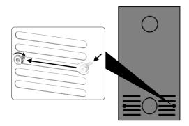
1) Guide the power cable with plug through the rear panel and fasten it as per the picture.
