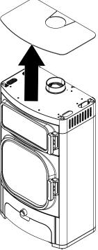
Fig. 48: Removing the hob
