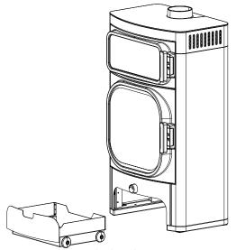
Fig. 30: Inserting the log drawer
