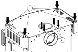
Fig. 14: Setting rubber cushions and adjusting screws
