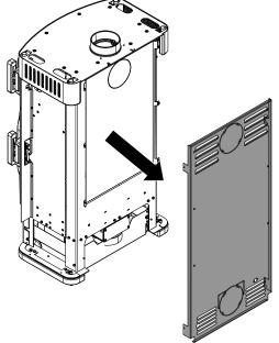
Fig. 59: Detaching the rear panel
