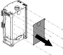
Fig. 11: Detaching the radiation protection
