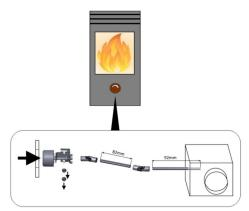
Fig. 34: Remove rotary control unit
