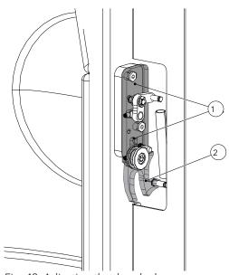
Fig. 42: Adjusting the door lock
