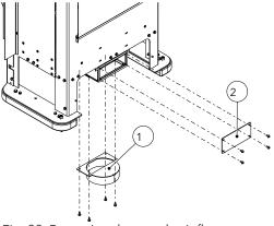
Fig. 28: Removing the supply air flange
