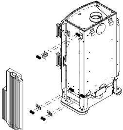
Fig. 22: Mounting HMS holder and HMS
