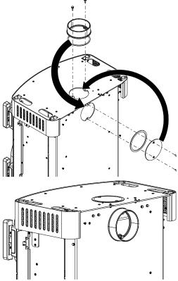
Fig. 13: Replacing cover and bracket
