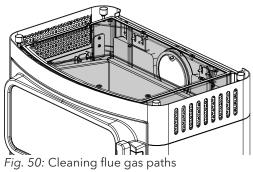
6) Undo all the screws from the lid and remove the lid.
