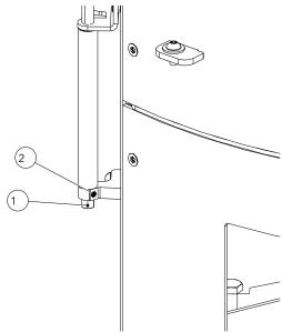
Fig. 41: Adjusting the closing pressure of the door
