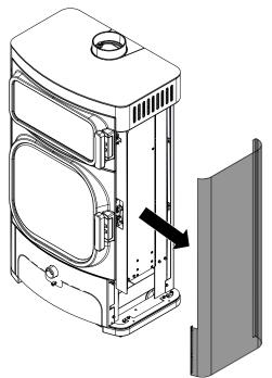
Fig. 57: Detaching the side cladding
