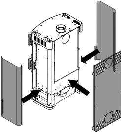
Fig. 18: Mounting the rear panel and side cladding
