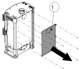
Fig. 17: Mounting the radiation protection
