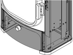
Fig. 33: Mounting the side cladding
