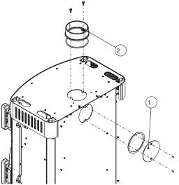
Fig. 12: Remove cover and bracket
