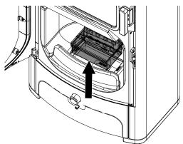
Fig. 54: Removing and emptying the ash box
