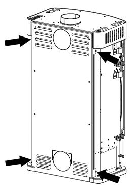
Fig. 58: Undoing the screws on the left and right of the rear panel
