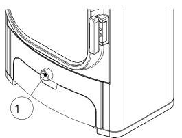
Fig. 45: Primary/secondary air controller
