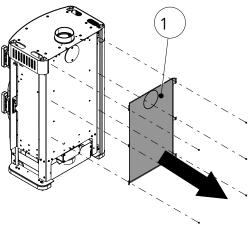
Fig. 20: Removing the radiation protection
