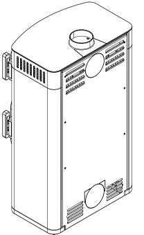
Fig. 24: Attaching side cladding, lid and hob
