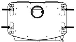
Fig. 55: Undoing the screws from above
