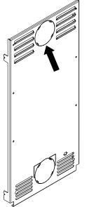
Fig. 10: Removing the perforated cut-out
