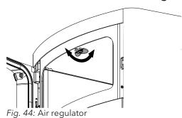
An air regulator is located inside the baking compartment. You can use this air regulator to have the moisture drawn out of the baking compartment.
