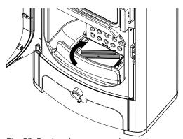
Fig. 52: Putting the cover on the ash box
