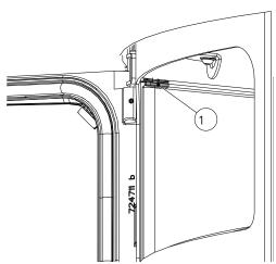
Fig. 27: Holders for Keramott bricks
