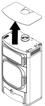
Fig. 9: Removing the hob
