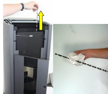
Fig. 81: turbulator removal and cleaning
