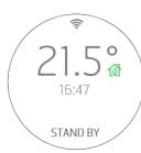
When the room temperature reaches the set temperature and all the other parameters are also respected (see the next paragraph), the equipment switches off and the display indicates the room temperature, the current time and the STANDBY indication to indicate the standby mode, which allows the product to turn on again as soon as the temperature drops below the set threshold or if the intended temperature in the room increases.
