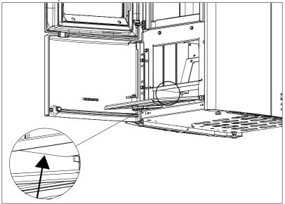
Then remove the upper calorite plate "J" to do this open the firebox door, hold the top of the calorite plate "J" and lift it upwards, tilt it to the right or to the left in order to release it from the supports and remove it.
