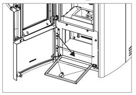
Attention! When cleaning is completed, remember to place back the ash pan "P", close again all doors ("I", "R", "F"), insert the brazier and the ash gate "S".
