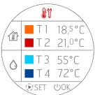
By pressing the SET key, the first temperature (T1) becomes RED and the eye keys can be used to proceed with the modification in steps of 0.5°C. As usual, a prolonged pressure of the eye keys results in temperature variations in higher steps, following the same philosophy of the temperature changes on the panel.
