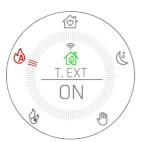
ON indicates that the thermostat contact is CLOSED and there is a power demand and therefore the stove will run at maximum power until the temperature is reached and it will then turn off according to the START&STOP logics.
