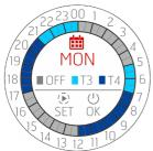
If T3 and T4 temperatures are selected, the summary display simply changes colour and the key is updated since it is not possible to set the chrono slot where both the AIR temperatures (T1 and T2) and the WATER temperatures (T3 and T4) are present simultaneously
