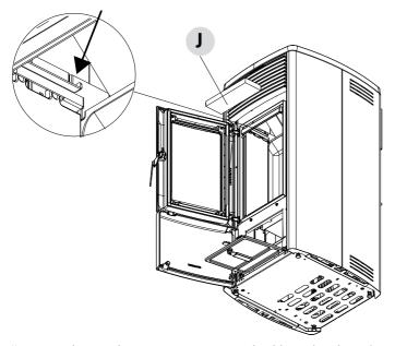
Use a vacuum cleaner nozzle to vacuum up any remaining ash and dust on the exchanger (see arrow). Then thoroughly clean the lower exchanger, replace any gaskets if needed, and reassemble.
