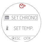
To set the temperatures of SETT1 – T2 – T3 – T4 (T3 and T4 only for Hydro stoves) you must enter the menu **SET TEMP**. selecting the item with the  $\oplus$   $\ominus$  keys and confirming with the  $\circlearrowleft$  OK key.
