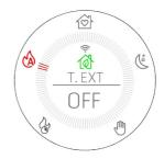
OFF indicates that the thermostat contact is OPEN and there is NO power demand and therefore the stove will run at minimum power until the START&STOP INPUT time is satisfied.
