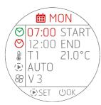
At the start of programming, the first **START** field is coloured red. Use the  $\oplus$   $\ominus$  keys to adjust the START time of the chrono slot.
