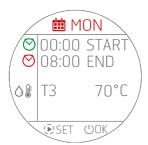
With respect to AIR products, there are fewer possible settings which are only START, END and the water temperature in the puffer/boiler.
