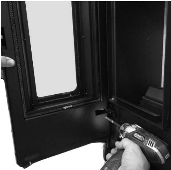
Fig. 84 - Loosen the screw
