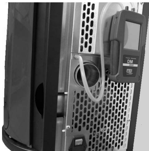
Fig. 54 - Digital pressure switch connection
