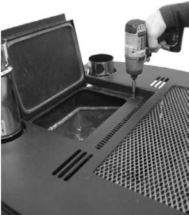
Fig. 41 - Upper screws removal
