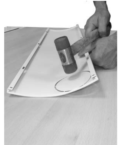
Fig. 38 - Open the hole (Sfera 3 Plus model)
