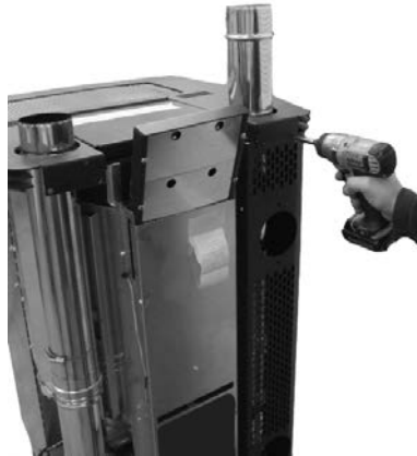
Fig. 42 - Backward screws removal
