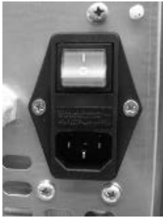
Fig. 53 - Electric socket with master switch
