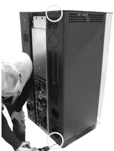
Fig. 93 - Rear screws removal
