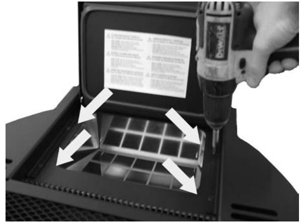
Fig. 81 - Cover 2 screw removal
