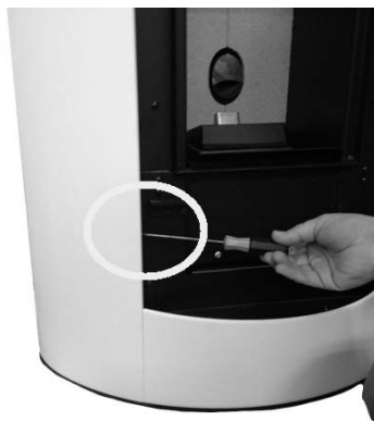
Fig. 87 - Loosen the bottom screw
