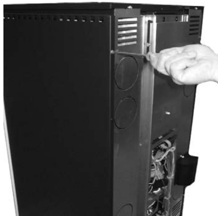
Fig. 75 - Removing the rear screw
