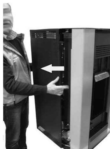
Fig. 94 - Remove side panels
