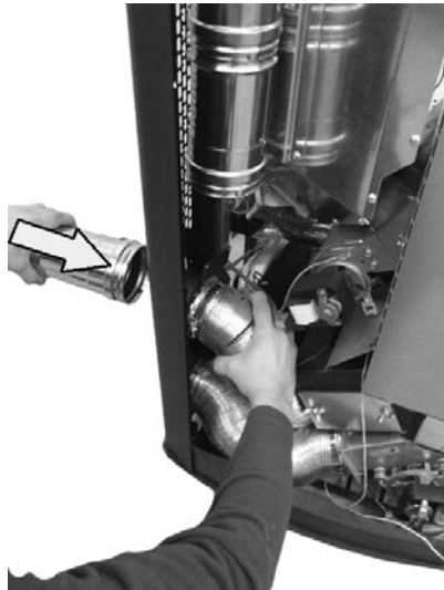
Fig. 65 - Pipe positioning for ducting
