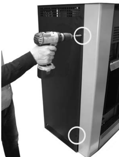
Fig. 92 - Remove the side screws
