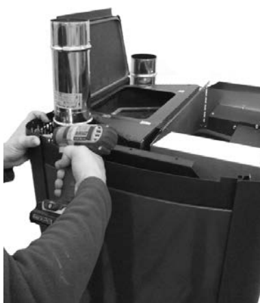
Fig. 90 - Removing the upper curve profiles
