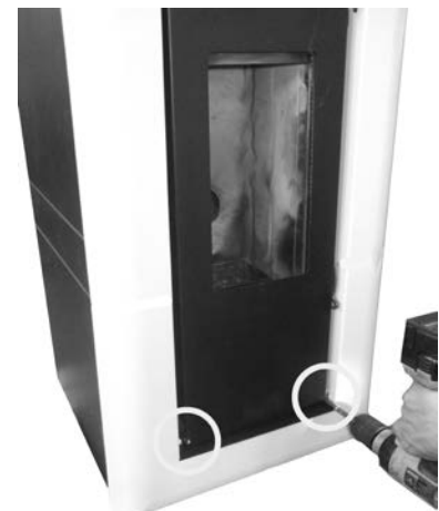
Fig. 32 - Frontal panel fixing
