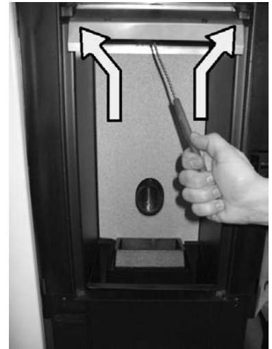
Fig. 97 - Clean both the ducts
