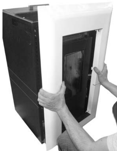
Fig. 31 - Frontal panel position
