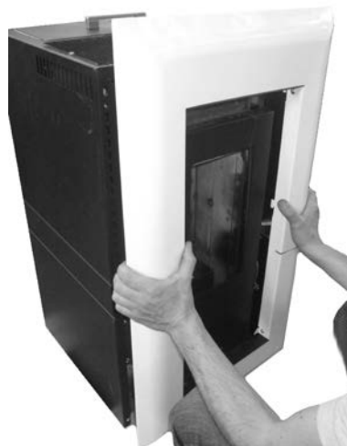
Fig. 25 - Frontal panel position
