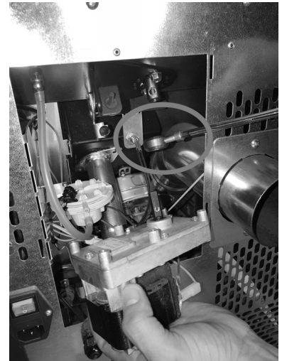
Fig. 80 - Gear motor removal
