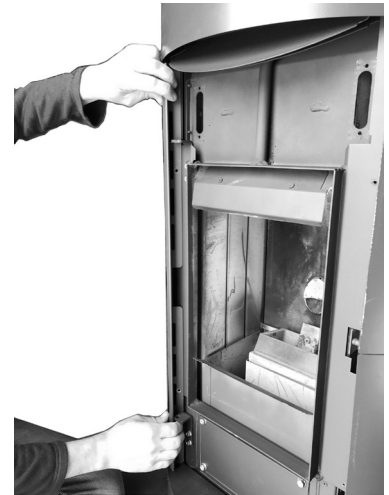
Fig. 66 - Front profile removal (rh and lh).
