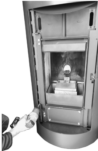
Fig. 65 - Profile screws removal (rh and lh).
