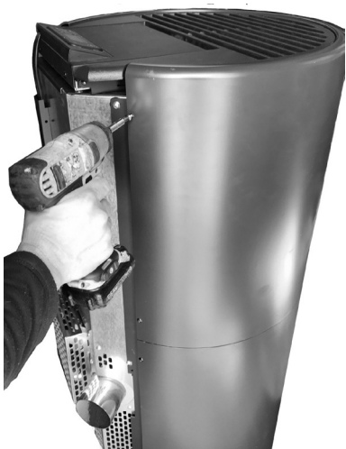
Fig. 67 - Rear screws removal
