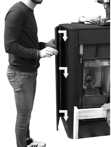
Fig. 47 - Slide the panel on
