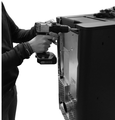
Fig. 48 - Remove the screws
