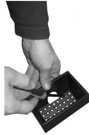
Fig. 29 - Burning pot cleaning
