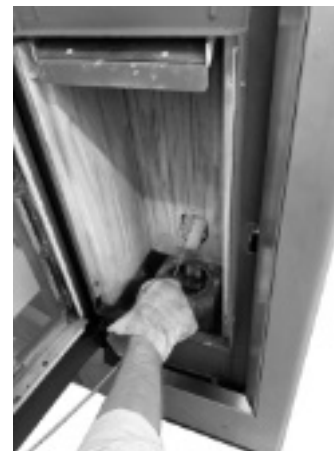
Fig. 34 - Cleaning with a brush
