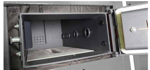
Fig. 14: Boiler wall / primary air openings
