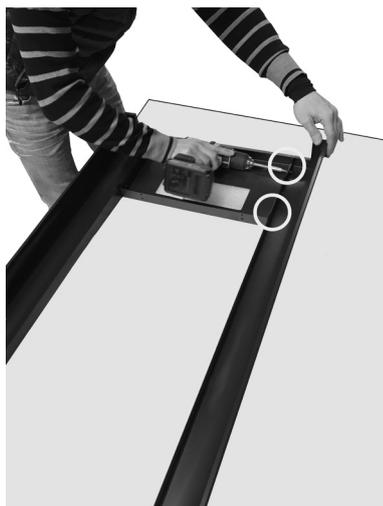
**Fig. 21 - Secure the strut**
