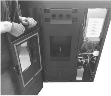
**Fig. 41 - Remove the door**
