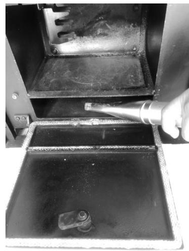
**Fig. 85 - Vacuum out the ash**
