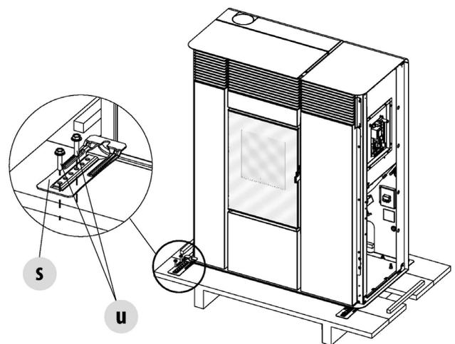
**Fig. 3 - Remove the fastening brackets**
