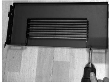
**Fig. 28 - Remove the grid**
