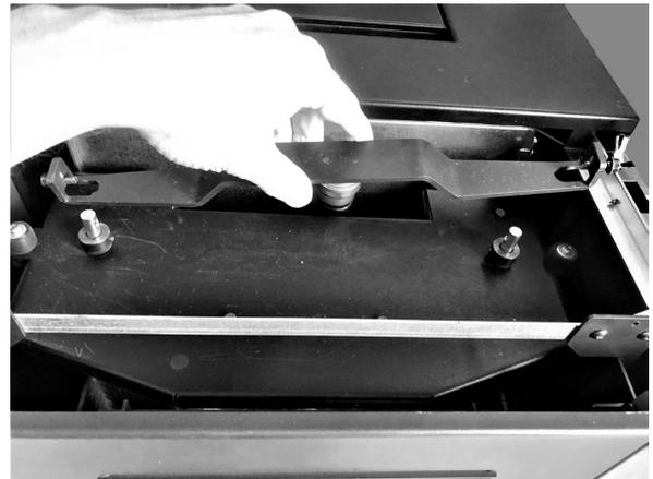
**Fig. 89 - Remove the handle**
