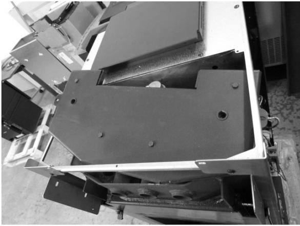
**Fig. 92 - Remove the cover**
