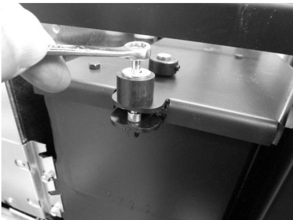
**Fig. 90 - Unscrew screw using 8 mm spanner**
