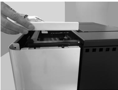
**Fig. 51 - Placing the top panel**
