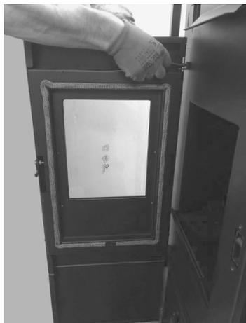
Fig. 19 - Removing the screws
