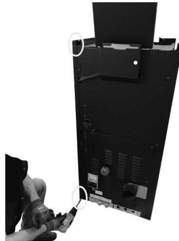
**Fig. 50 - Secure the rear side panel**
