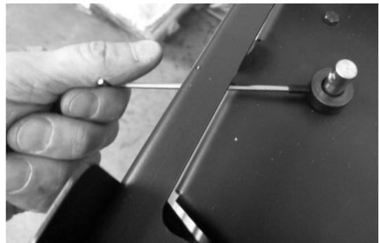
**Fig. 91 - Unscrew screw using 2.5 mm spanner**
