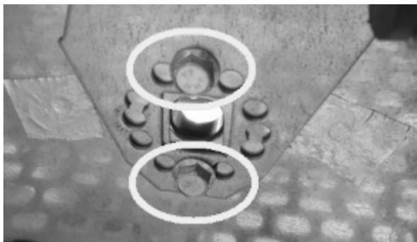
*Fig. 96 - Remove the screws*
