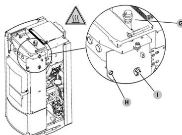
**Fig. 63 - Manual bleed valve (located under the top) (Idro Prince³ 16-23-23 H2O, Aquos³ 16-23-23 H2O, Idron 16-22 Airtight, Hidrofire 22.8)**
