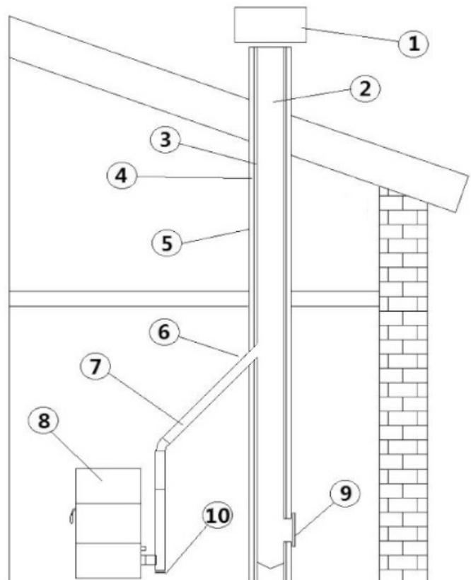
Fig. 5 - Chimney components
