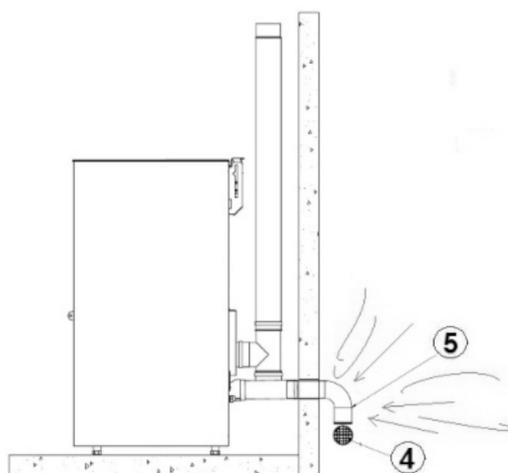
Fig. 11 - Air inlet for sealed-chamber installation
