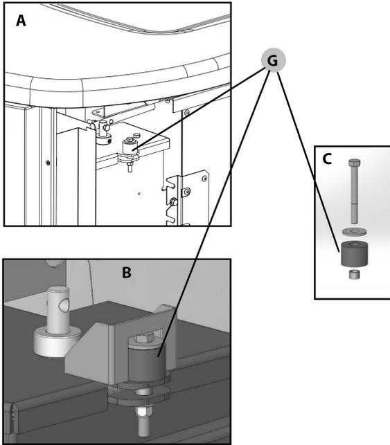
**Fig. 86 - Rubber spacer**
