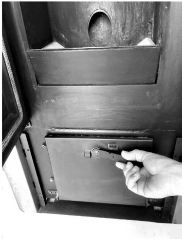
Fig. 79 - Remove the screws
