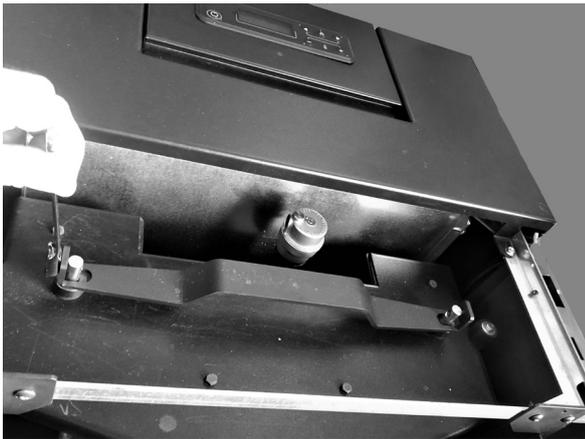
**Fig. 88 - Unscrew screw using 8 mm spanner**
