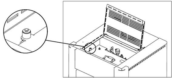
**Fig. 87 - Rubber spacer**
