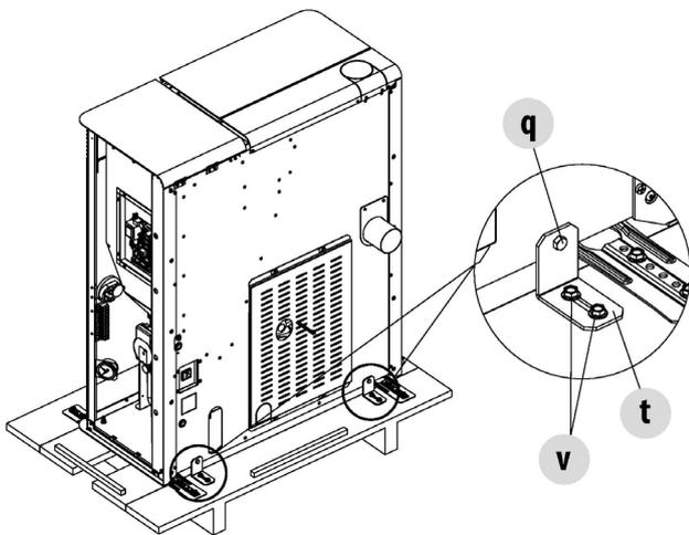
**Fig. 2 - Remove the fastening brackets**
