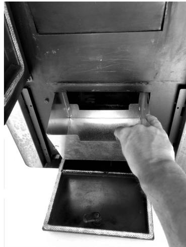
Fig. 80 - Remove the inspection cap
