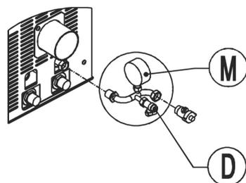
**Fig. 62 - Terminal with filling valve (D) and pressure gauge (M)**
