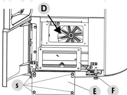
Fig. 77 - Lower compartment cleaning
