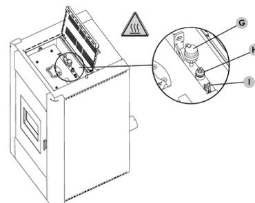
**Fig. 64 - Manual bleed valve (located under the top) (Idro Prince³ 30-30 H2O)**
