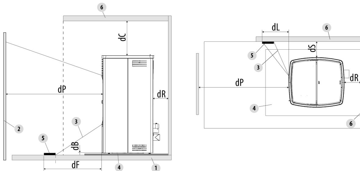
Fig. 14 - Safety distances from combustible material.
