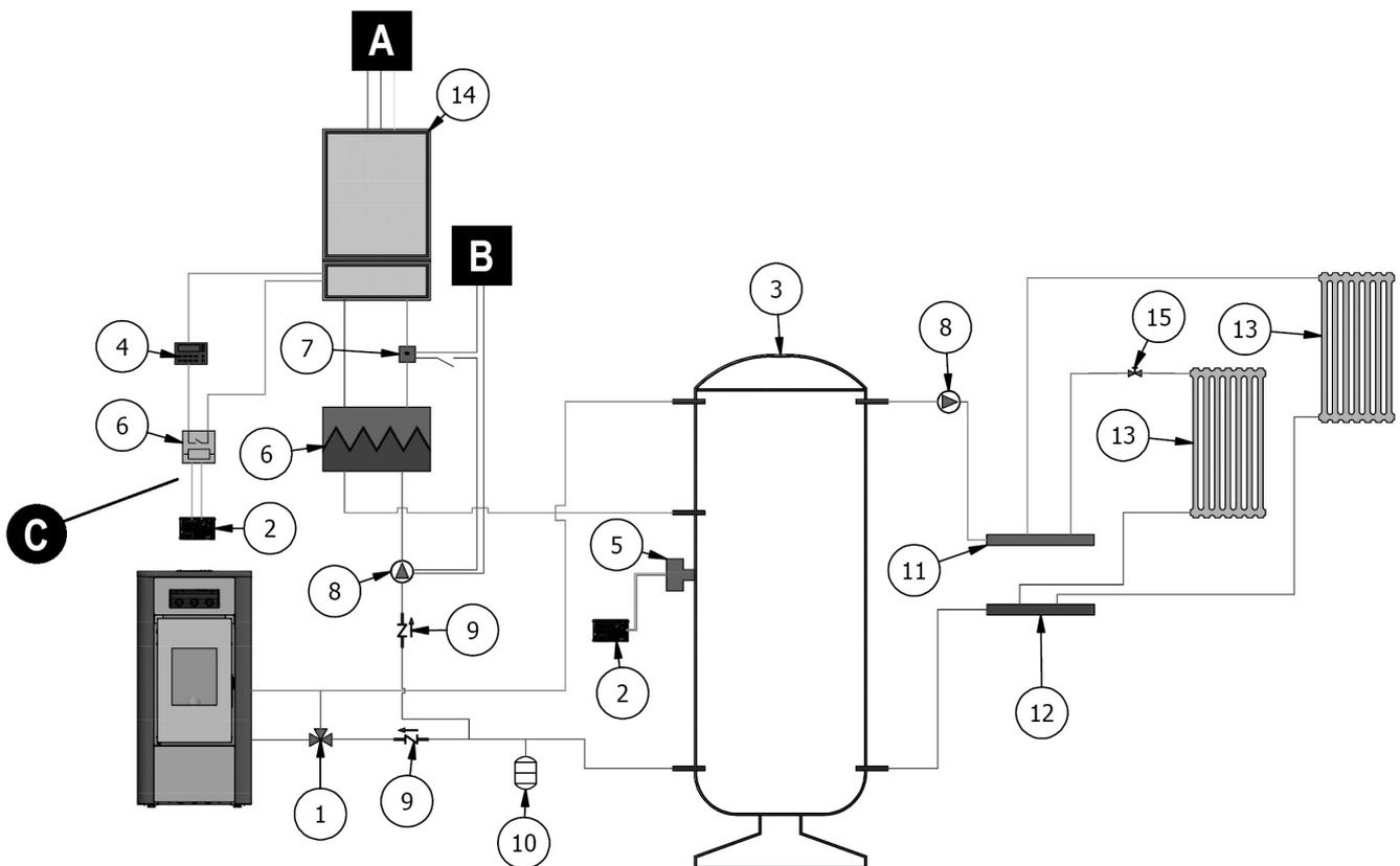
Fig. 71 - Configuration with storage tank and auxiliary wall-mounted boiler
