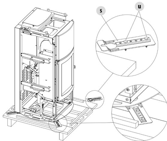
**Fig. 1 - Remove the fastening brackets**
