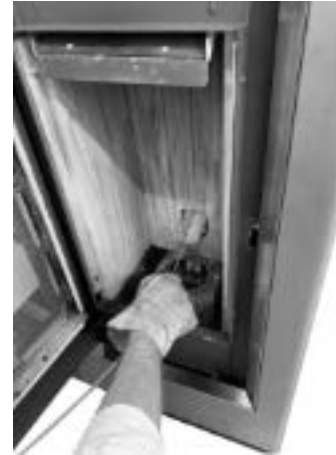
Fig. 36 - Cleaning with a brush
