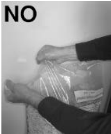
Fig. 24 - Wrong opening of the pellets bag
