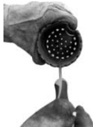
Fig. 34 - Burning pot cleaning
