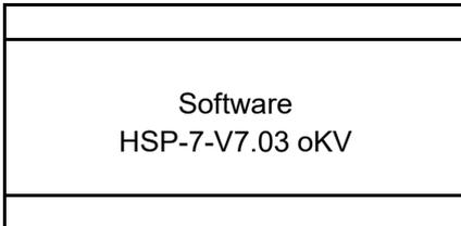
As soon as the mains plug is connected, the software version appears on the display for approx. 7 seconds, E.g.:
