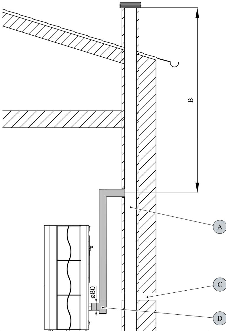
**Figure 1: Connection to the chimney:**
